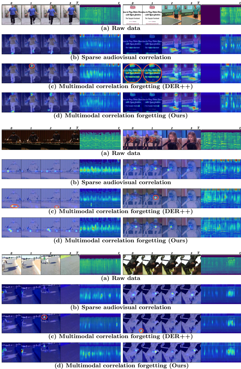
Figure 2.16: Visualization of cross-attention maps. (a) Examples of raw data pairs. We visualize cross-attention maps of the pairs in (b). The closer the color is to red, the higher the attention score. While the baseline model using DER++ attends to entirely different parts as can be seen in (c), our method attends to a similar part even after being trained on two additional tasks as presented in (d). The wrong attention region is marked in an orange circle.
